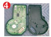
CAREFULLY SEPARATE THE TWO HALFS, MAKING SURE NOT TO DROP THE INSIDES. THEY WILL FALL OUT.
