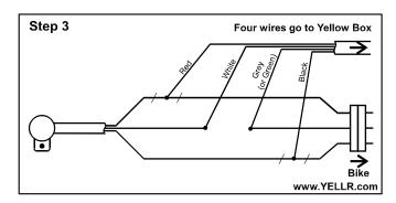
You must connect the Yellow Box wires exactly as shown above, or your speedo may not work properly. Carefully **compare your work** to the Step 2 and Step 3 pictures, and with the before and after diagrams on page 1.
